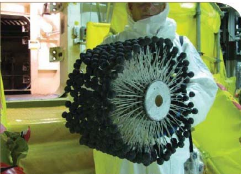
The Flex-Hone, used for decontamination of large-bore water pipes at a nuclear power plant. The tool is considered disposable so it requires no decontamination after use in a radioactive pipe. Photo, Brush Research.
